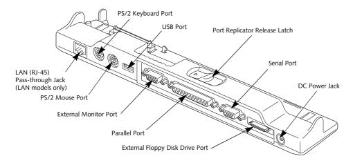
Figure 4-12 Port Replicator back panel (LAN model)
